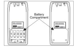
For the best service life, use nickel cadmium rechargeable or alkaline batteries in the receiver.
